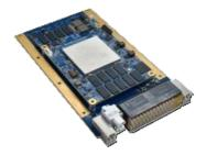
**3U VPX Module**: **iW-RainboW-G35V**, comprises of the Zynq UltraScale+ MPSoC SOM and a 3U-VPX Carrier board. It features 8GB DDR4 RAM with ECC and expandable on-board flash storage, ensuring reliable performance. This 160mm x 100mm module rugged plug-in module is tailored for high-speed video and data processing, perfect for military and aerospace applications.
