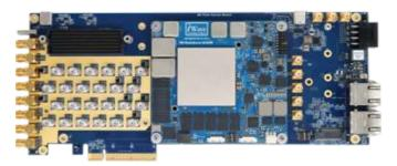
The RF-PCIe Carrier Board is integrated with all necessary on-board connectors to validate the features of Zynq UltraScale+ RFSoC (ZU49/39/29DR) SOM, and supports 16 Channel RF-DACs at 10Gsps and 16 Channel RF-ADCs at 2.5Gsps. The card is equipped with 8GB DDR4 RAM and M.2 NVMe slots for expanded storage options, and PCIe Gen 1, 2, and 3 compliant interfaces and multiple SMA connectors for easy validation, with FMC+ interface.
