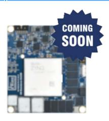
We will shortly be launching the ZU48/47/43/28/27/25DR powered SoM, that is built to support high-speed 8 x ADC Channels up to 5Gsps and 8 x DAC Channels up to 9.85Gsps.
