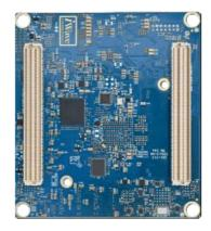
The ZU49/39/29DR RFSoC powered SoM supports 16 x ADC Channels up to 2.5Gsps and 16 x DAC Channels up to 10Gsps. The SoM supports 2 x 400 Pin board to board connectors that support a multitude of interfaces, including 16 x PL-GTY High Speed Transceivers with speeds up to 28.21Gbps.
