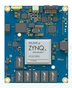
Xilinx Zynq UltraScale+ SoC based System On Module features the Xilinx's Zynq UltraScale+ SoC CG/EG devices with FFVC900 Package. The MPSoC Supports Quad/Dual Cortex A53 up to 1.5GHz with programmable logic cells ranging from 469K to 747K. The SOM supports high speed connectivity peripherals such as PCle, USB3.0, SATA3.1, Display port, Gigabit Ethernet through GTR high speed transceivers from MPSoC.
