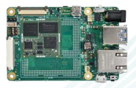
The STM32MP13x SBC integrates ST Microelectronics STM32MP13x: Cortex®-A7@up to 1 GHz, 10/100/1000 Mbps Ethernet PHY, and 18-bit RGB display support. The STM32MP13x-based SBC is aimed at applications mainly focusing on machine learning, NPU and vision systems, advanced multimedia, and industrial automation with high performance. With its 85mm x 56mm small form factor, the SBC is packed with all the necessary on-board connectors.
