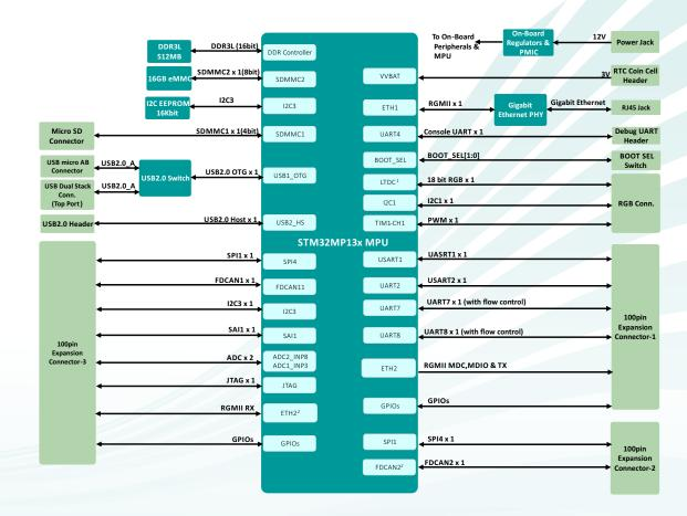
Note: STM32MP135,STM32MP133 & STM32MP135 CPUs can be supported. By default, the CPU used is STM32MP135. 1 RGB display will be supported only in STM32MP135 SOC. 2 Not supported in STM32MP131 SOC.
