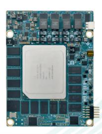
Intel Agilex 7 R31B/R31C SoC FPGA based System on Modules features.
