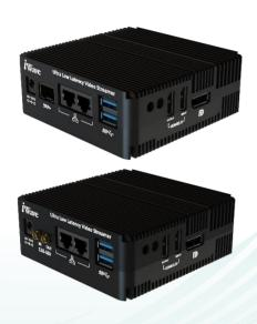
iWave's ULL Streamer meets the real-world challenges and dispense a streaming solution for ultra-low Latency streaming. The applications of the device are for live video streaming and embedded vision. It is capable of compressing and decompressing video streams simultaneously at resolutions of up to 3840 x 2160 pixels at 60frames per second (4K UHD at 60 Hz).
