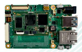
The Renesas RZ/G2UL or RZ/A3UL or RZ/FIVE based SBC definition targeting application that require low power, low costs, and high performance. The SBCs are used as building blocks for portable and stationary embedded systems. The core CPU and support circuits, including DRAM, boot flash, power sequencing, CPU power supplies and GbE are concentrated on the SBC.
