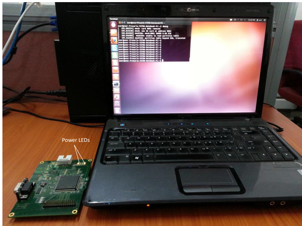
Figure 4: SD Memory Slave IP test setup
