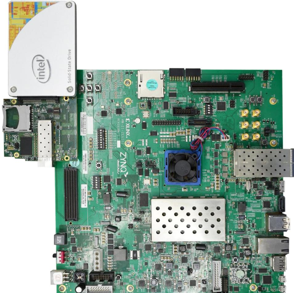
Figure 1: SATA 3.0 Host Controller setup
