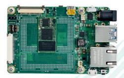
The STM32MP13x SBC integrates ST microelectronics STM32MP131/ STM32MP133/ STM32MP135: Cortex®-A7@up to 1 GHz, Support 10/100/1000 Mbps Ethernet PHY. The STM32MP135-based SBC is aimed at applications mainly focusing on machine learning, NPU and vision systems, advanced multimedia, and industrial automation with high performance. With its 85mm x 56mm form factor, the SBC is packed with all the necessary on-board connectors.
