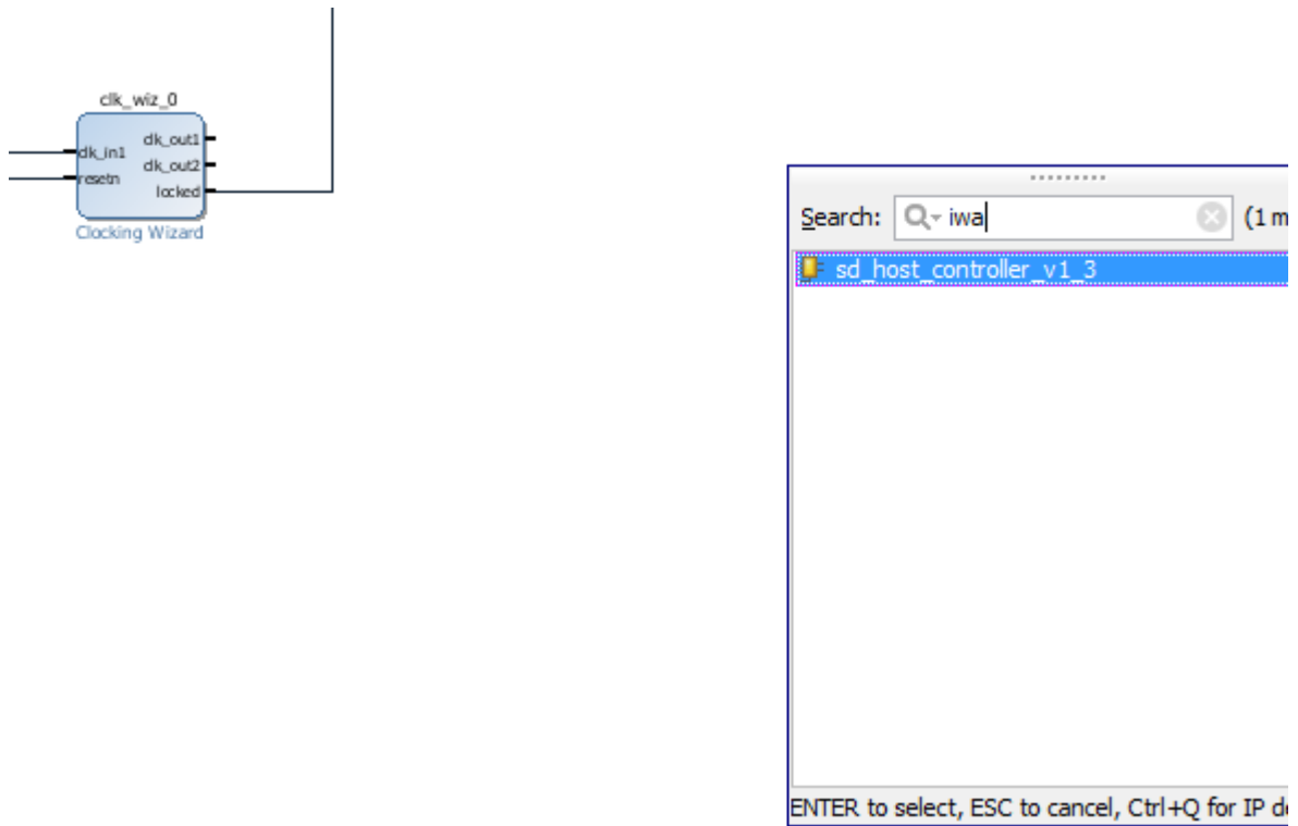
Figure 7: Step#5 to instantiate the iWave SD Host Controller IP in Design
