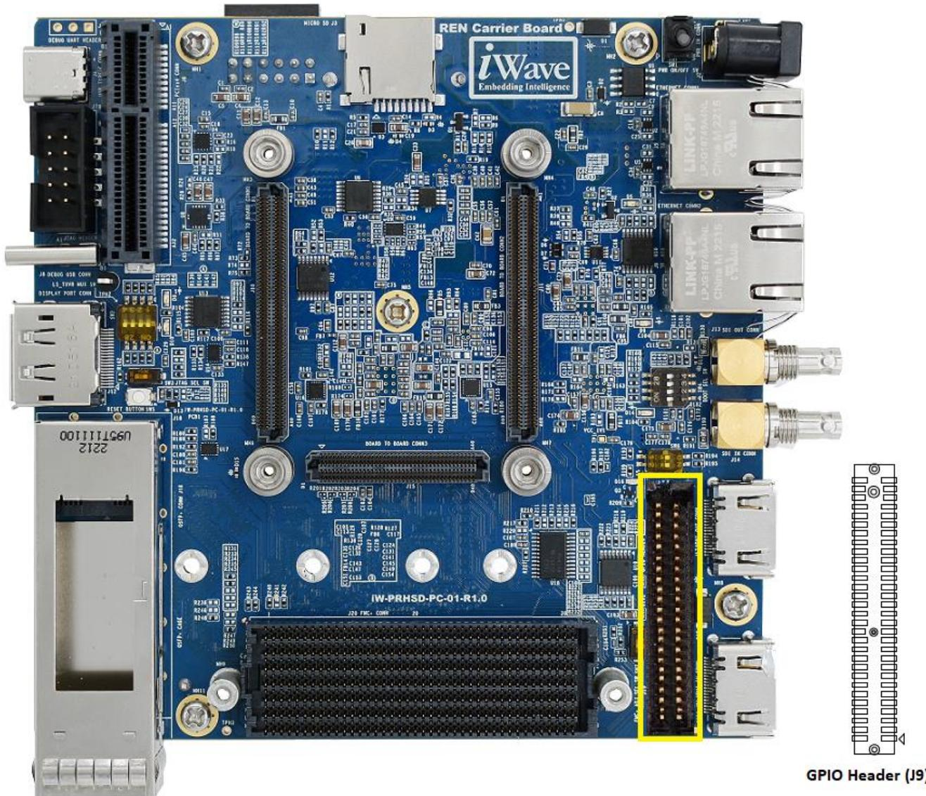
Figure 8: GPIO Header
