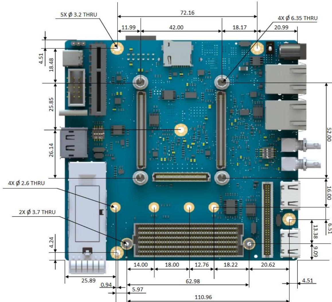
**Figure 23: Carrier board Mechanical dimension – Top View**
