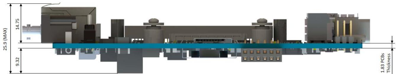
**Figure 24: Carrier board Mechanical dimension – Side View**
