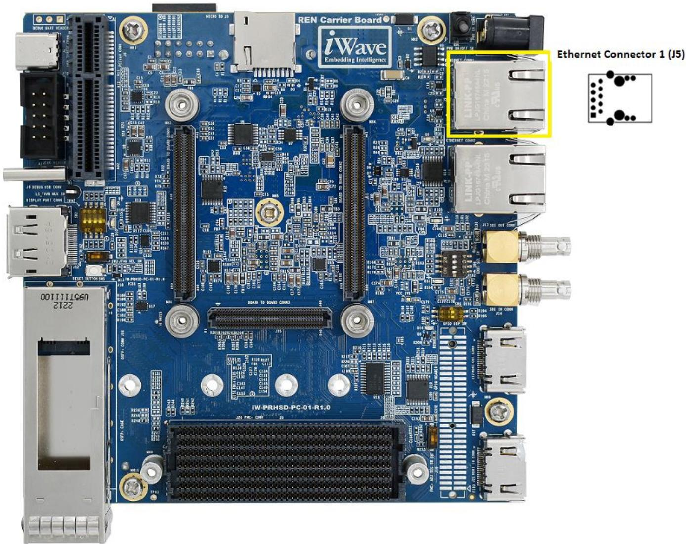
Figure 4: Gigabit Ethernet Connector1
