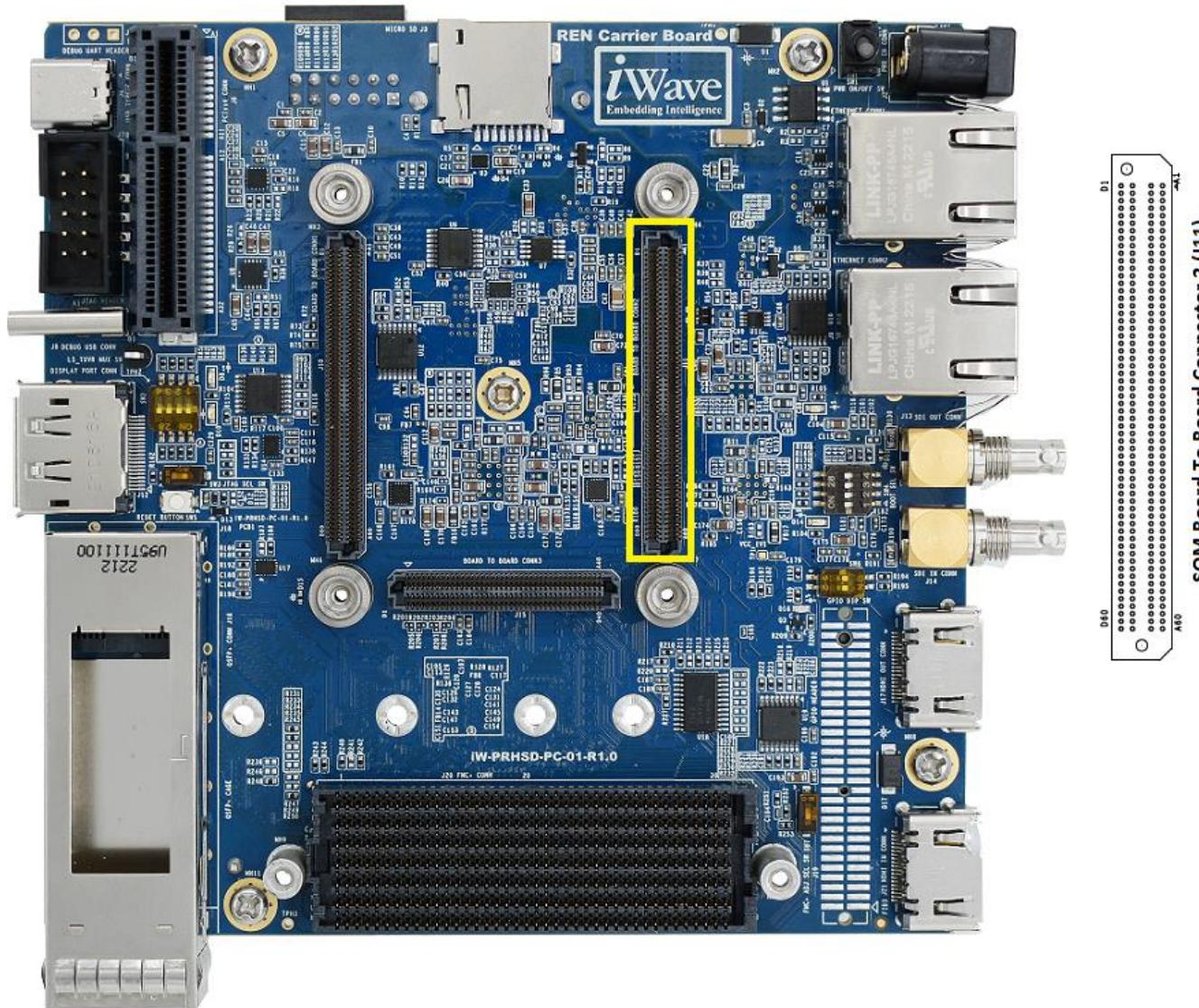
**Figure 3: Board to Board Connector 2**
