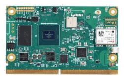
The <u>i.MX 8M Plus</u> development kit and software board support packages provided by iWave, helped the team to jumpstart the project by offloading several complexities involved in the design cycle. The i.MX 8M Plus applications processor is powered by a multi-core ARM Cortex-A53 processor operating at a maximum frequency of 1.8GHz, Cortex-M7 for real-time control and high industrial reliability with DRAM and inline ECC.
