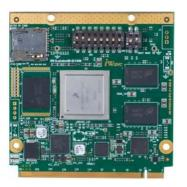
The <u>i.MX 6 System on Module</u> is available in a modular and compact Qseven form factor (70mmx70mm) with support for wide operating temperatures. Its power-efficient ARM Cortex A9 processor, combined with advanced Linux and Android firmware and support for all standard interfaces such as Gigabit Ethernet, PCIe, SATA 3.0, USA 2.0, and GPIOs, delivers rich media content like animations, effects, static images, and HD video combined with bus operational data.
