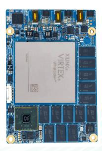
Virtex Ultrascale+ FPGA System On Module supports Virtex Ultrascale+ FPGA and ARM Cortex A7 processor. The SOM features FPGA with programmable logic cells up to 3780K and Power-efficient 32-bit Dual Arm Cortex-A7 processor running up to 1.2 GHz.
