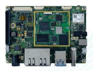
The i.MX 93 Pico ITX SBC integrates NXP's i.MX 93 offerings Dual Cortex A55 @ 1.7GHz, NPU with up to 0.5 TOP/s, IEEE 802.11 a/b/g/n/ac/ax Wi Fi + Bluetooth 5.3+ IEEE802.15.4 module, 10/100/1000 Mbps Ethernet PHY, MIPI-DSI, LVDS, MIPI CSI Camera support and GNSS Module.
