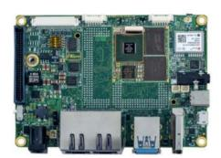
The i.MX 8XLite Pico ITX SBC integrates NXP's i.MX 8XLite offerings Dual/ Solo Cortex A35 @ 1.2GHz and 1 x Cortex-M4F cores with on board Dual 10/100/1000 Mbps Ethernet PHY.
