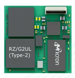
The Renesas G2UL or G2LC SoC based LGA modules are designed as per the Open Standard Module<sup>TM</sup> Size-S Specification (OSM). This module can be integrated with any one of the two Renesas SoCs - G2UL or G2LC SoCs.
