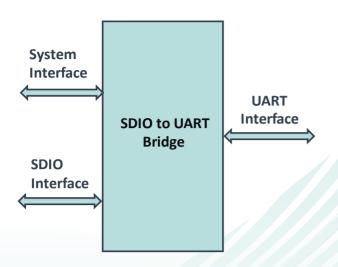
iW-SDIO to UART bridge is a IP core which converts SDIO slave to UART bus interface. SDIO Slave controller facilitates the design of SDIO cards and reduces the development time. By using this IP core, customers no longer need to spend time on handling the SD bus protocol since such function is provided by the core.
