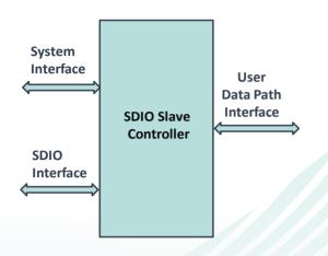
SDIO Slave controller facilitates the design of SDIO cards and reduces the development time. By using this IP core, customers no longer need to spend time on handling the SD bus protocol since such function is provided by the core.
