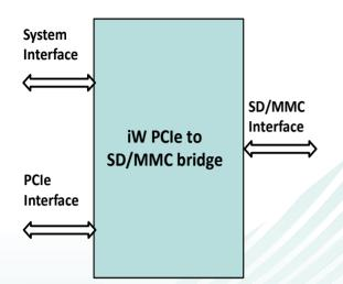
iW-PCle to SD/MMC Bridge is the IP core which converts the PCle to SD or MMC bus interface. The interface towards the SD or MMC card is realized by the SD or MMC protocol implemented in the controller.
