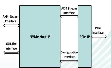
The NVMe IP core is compliant with NVM Express base specification revision 1.4 that performs memory transfer to or from the NVMe storage like SSDs. The IP core is designed to handle NVMe protocols without the need for external DDR memory via a PCIe interface. It is ideal for applications that require large storage capacity with high performance and is available with flexible vendor-specific PCIe IP to access SSD.
