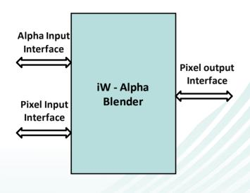
iW- Alpha Blender is used when two video sources have to be viewed at the same time. It is a process of combining an image with a background to create the appearance of partial or full transparency. This core can be easily integrated into video, medical, commercial and entertainment kind of applications which use LCD display.
