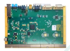
iWave's Cyclone V FPGA based 6U cPCI form factor conversion card is a rugged standalone module used for ARINC 818 to DVI conversion, DVI to ARINC 818 Conversion, ARINC 818 Mux as well as ARINC 818 Duplicator either on front panel or via cPCI back panel.
