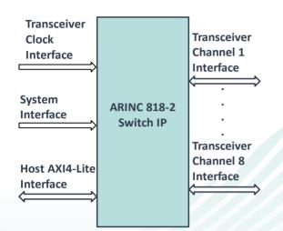
Since a vast portion of the newer applications of the ARINC 818-2 have several displays with many channels of ARINC 818-2 (4 to 8 Channels), switching has turned out to be more imperative. iW ARINC 818-2 Switch IP core is compatible with the ARINC 818-2 specification.
