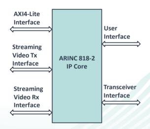
iW ARINC 818-2 IP core is compatible with the ARINC 818-2 specification. The ARINC 818-2 IP core can be implemented on any transceiver based FPGA. It can be used for both transmitand-receive applications. This core supports simple streaming interface which can be integrated with video & image processing IP cores supported by the FPGA vendors.
