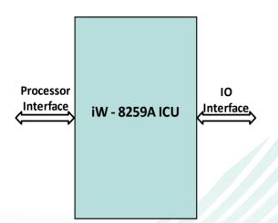
iW-Interrupt Controller is designed to transfer the interrupt with highest priority to the CPU, along with interrupt address information.
