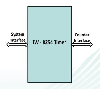
iW- Programmable Timer used for timing control applications in microcomputer systems. The design is capable of generating accurate time delays under software control. Three independent 16-bit counters are supported which can be configured to operate in one of the six operating modes supported
