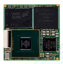
The i.MX 8XLite SoC based LGA Module is designed as per the Open Standard Module<sup>™</sup> specification (OSM). It integrates NXP's i.MX 8XLite offerings Dual/Solo Cortex A35 @ 1.2GHz, advanced multicore processing with V2X acceleration supported by Arm® cores.
