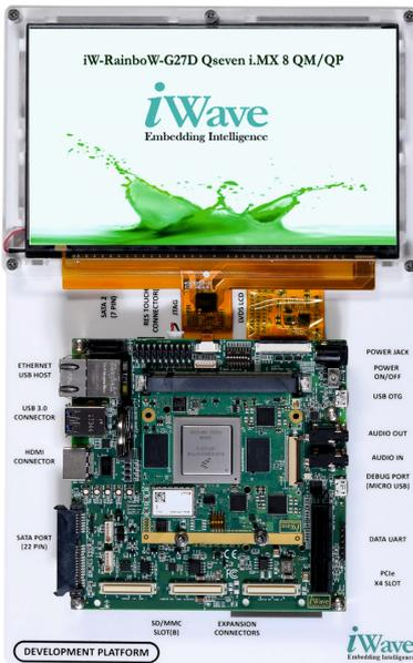
The i.MX 8 QM/QP (Quad Max/Quad Plus) Qseven Development platform combines the NXP i.MX 8 QM/QP application processor based Qseven SOM and iWave's Generic Qseven Carrier Card to offer maximum performance with higher efficiency for complex consumer, medical and industrial embedded computing applications. The board is highly packed with all necessary onboard connectors to validate i.MX 8 QM/QP SoC features to the fullest.
