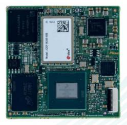
The i.MX 8M Plus SoC based LGA Module is designed as per The Open Standard Module<sup>™</sup> specification (OSM).It integrates NXP's i.MX 8M Plus offerings Quad/ QuadLite /Dual Cortex A53 @ up to 1.8GHz, NPU with up to 2.3 TOP/s, HDR capable Image Signal Processor (ISP) with IEEE 802.11 a/b/g/n/ac/ax\* Wi Fi & BT 5.0 module.
