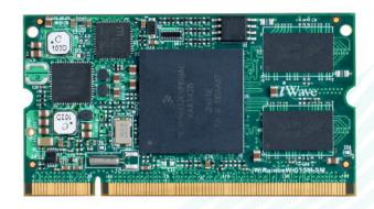
iWave's new i.MX6 Quad/Dual/Dual Lite/Solo based SODIMM module integrates all standard interfaces into a single board with ultra compact yet highly integrated platform that can be utilized across multiple embedded PC, system and industrial designs. It has got all the necessary functions that the embedded world demands.
