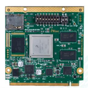
iWave Systems offers high performance Qseven SOM module based on NXP's i.MX6 ARM Cortex-A9 processor for faster and multimedia focused applications. With extreme peripheral integration, the CPU supports industry latest high-performance interfaces, such as PCle Gen2, Gigabit Ethernet, SATA 3.0, HDMI 1.4, SDXC, MIPI CSI/DSI and 64-Bit DDR3 interfaces.
