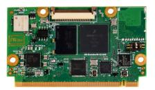
Extending the portfolio of i.MX8 System on Modules, the i.MX8M Mini / Nano Micro Q7 Module with a compact form factor of 70mm \* 40mm while powered with 4 \* Cortex - A53 Cores and 1 \* Cortex M4F Core is an ideal solution for space constrained solutions .
