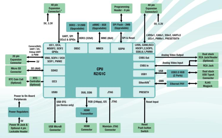
Note1: Since EtherAVB collision detection signal is multiplexed with VINO clock signal in CPU, EtherAVB collision detection feature is not supported by default. Note2: 40 Pin Expansion Connector1 pinout is compatible with RaspberryPi Connector.
