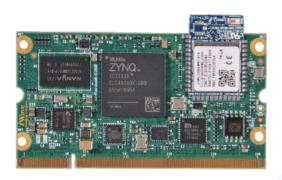
Xilinx Zynq 7000 SoC based System On Module (SOM) features the Xilinx Zynq 7000 series SoC with Dual Cortex A9 CPU @ 866MHz, 85K FPGA logic cells and up to 120 FPGA lOs. The SOM is equipped with on-board QSPI flash, eMMC, DDR3 RAM, Wi-Fi, BT and Gigabit Ethernet. This SOM is suitable for various industrial, embedded computing and medical applications.
