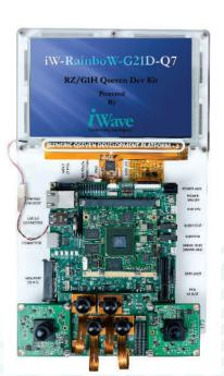
iWave's RZ/G1H development board incorporates RZ/G1H Qseven SOM which is based on Renesas' high performance RZ/G1H Quad ARM Cortex A15 MPU and the carrier board with optional 7" capacitive display kit. The development board can be used for quick prototyping of various applications targeted by the RZ/G1H processor. With the 120mm x120 mm Nano ITX size, the kit is highly packed with all the necessary on-board connectors to validate the RZ/G1H MPU features.
